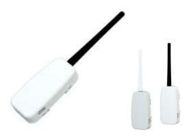
The Lora Low cost single channel base station can be use in private network to make the link between IOT Lora based devices to internet.
